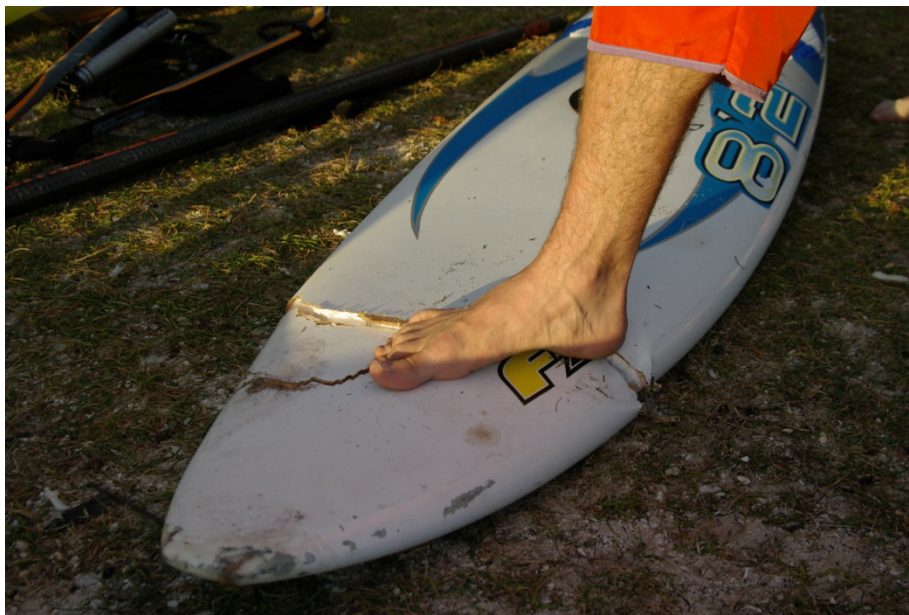
Fig. 8 Complete nose damage due to impact load
