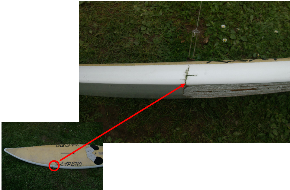
Fig. 19 Complete bottom fracture due to hard nose dive
