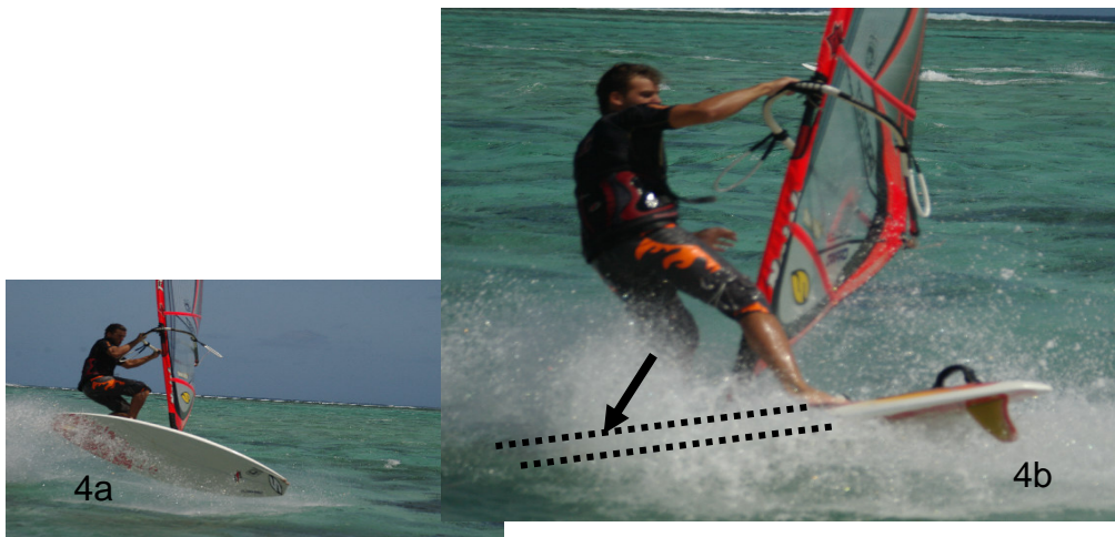
Fig. 4 "Willy Skipper": impact load on the nose part
