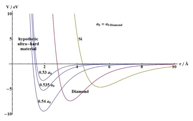
Fig. 8: Potential for Diamond, Silicon and three rather impossible hypothetic ultra-hard material with fcc-structure.
