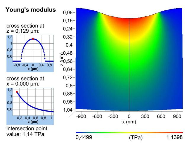
Fig. 4: Distribution of Young's modulus as result of hydrostatic stress underneath the indenter. Boundary conditions see text.
