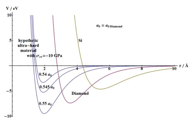
Fig. 9: Potential for Diamond, Silicon and a rather impossible hypothetic ultra-hard material with fcc-structure and an assumed biaxial intrinsic stress of -10 GPa.
