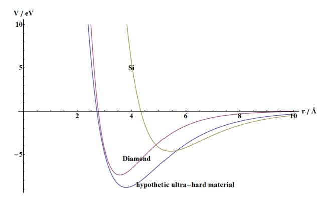
Fig. 5: Potential for Diamond, Silicon and a rather impossible hypothetic ultra-hard material.
