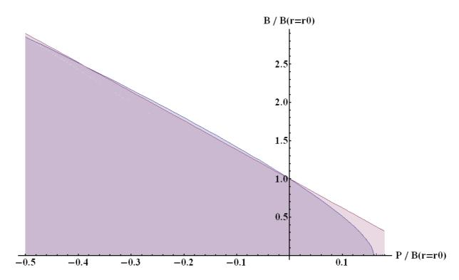
Fig. 2: Bulk modulus as function of the hydrostatic pressure evaluated from (1.2) and linear fit for supposed ultra-hard nano-composite TiN/a-Si<sub>3</sub>N<sub>4</sub> and nano-composite TiN/a-Si<sub>3</sub>N<sub>4</sub>/TiSi<sub>2</sub> with a much more reasonable parameter choice.
