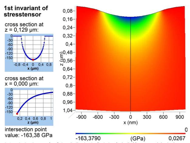
Fig. 3: First invariant stress for a fictive unloading situation (beginning of unloading) for a supposed ultra-hard material with yield strength short below 42 GPa. Boundary conditions see text.
