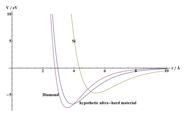
Fig. 7: Potential for Diamond, Silicon and a rather impossible hypothetic ultra-hard material with an assumed biaxial intrinsic stress of -10 GPa.
