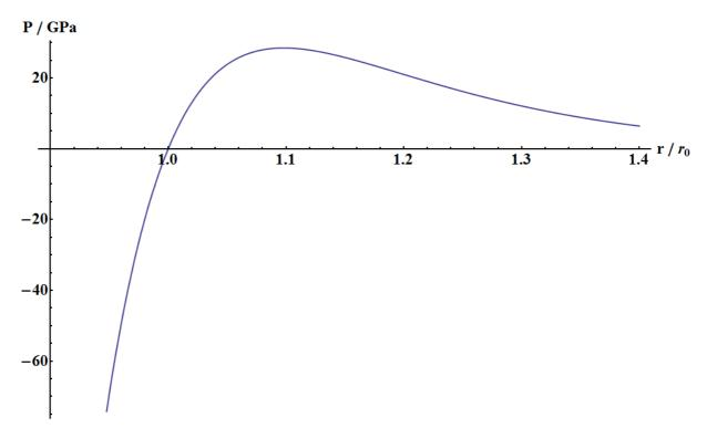
Fig. 6: Pressure as function of lattice constant over state of equilibrium for hypothetic ultra-hard material.
