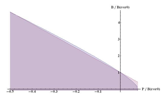
Fig. 1: Bulk modulus as function of the hydrostatic pressure evaluated from (1.2) and linear fit for supposed ultra-hard nano-composite TiN/a-Si<sub>3</sub>N<sub>4</sub> and nano-composite TiN/a-Si<sub>3</sub>N<sub>4</sub>/TiSi<sub>2</sub> with a parameter choice in favor of a highest as possible hardness. It must be pointed out however, that this choice of parameters is rather unphysical.
