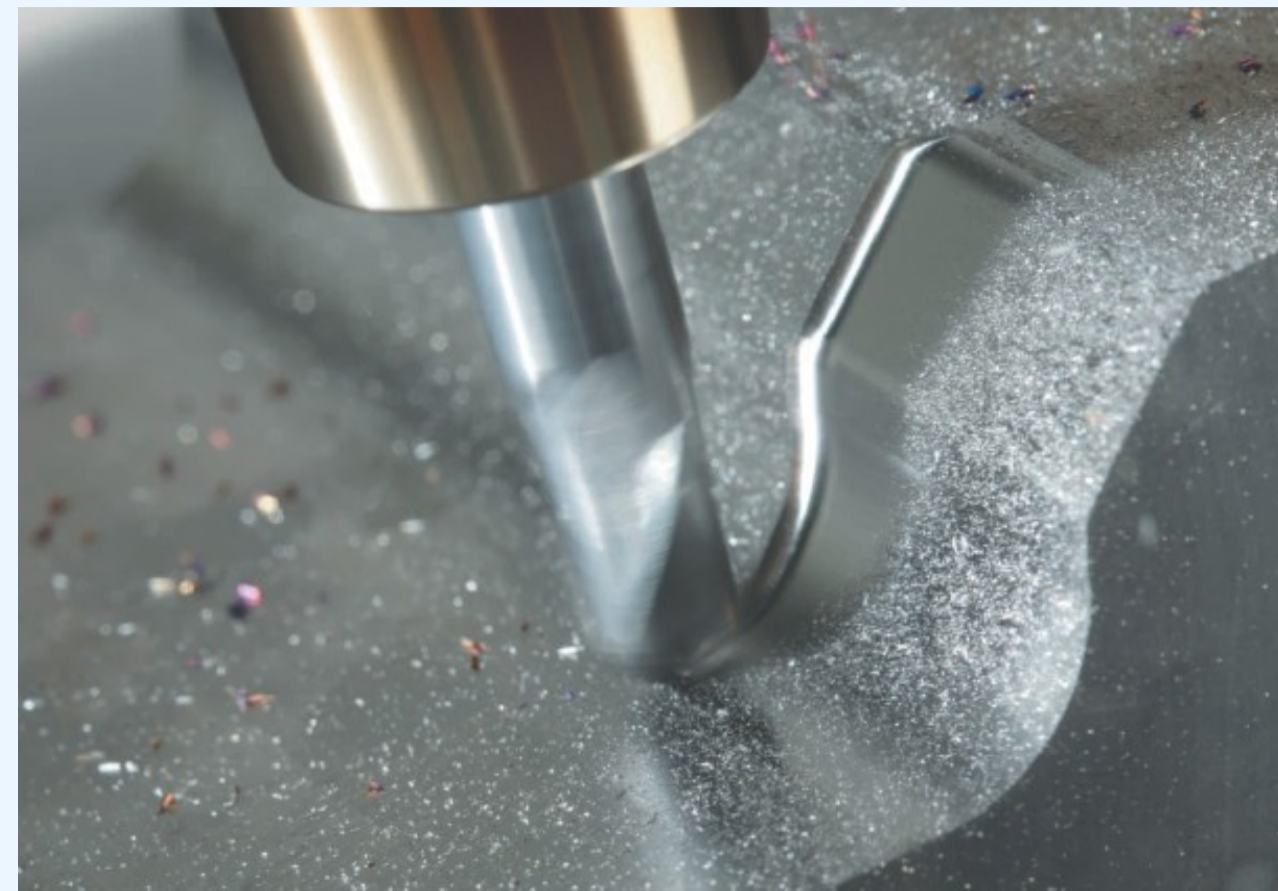
Fig. 2: Dry milling with coated tool
