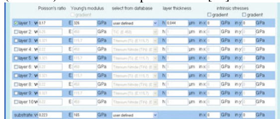
Fig. 5: Material definition page. Now we can type in the evaluated coating Young's modulus.
