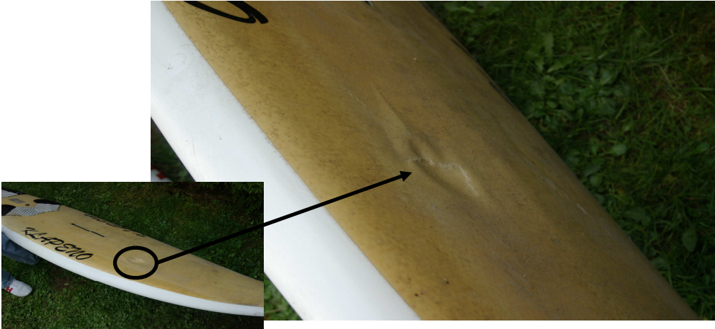
Fig. 6 Surface fracture damage due to impact load
