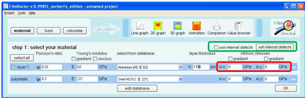
Fig. 1: Defining your material structure. Also possible: Simulating the intrinsic stresses correctly by the means of analytical interface defects. Next step is to load a series of indents with different maximum loads or just a so called multi-indent data set.
