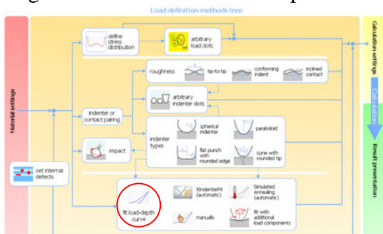
Fig. 4 Load definition for the simulation of mechanical contact situations with FilmDoctor® (www.siomec.de)
